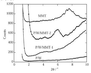
**Figure 1.**WAXD patterns of the polyol/water mixture (P/W), MMT and polyol/water-MMT mixtures (P/W/MMT-1 and P/W/MMT-2). P/W/MMT-1 and P/W/MMT-2 mixtures contain 7.65 and 14.9 wt.-% MMT, respectively, giving 5 and 10% wt.-% MMT in the final PU foams.
