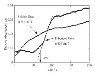
**Figure 4.** Phase-separation kinetics data showing the microphase-separation transition (MST) during the formation of unfilled foam (Fo). Data determined from the relative absorbances of hydrogen-bonded urea (1639 cm $^{-1}$ ) and soluble urea (1711 cm $^{-1}$ ) in forced-adiabatic FTIR spectra.
