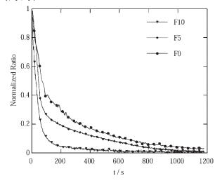
**Figure 3.**Normalised reaction kinetics data for the formation of unfilled foam (FO) and PLSN foams (F5 and F10). Data determined from the decay in isocyanate absorbances (2270 cm<sup>-1</sup>) in forced-adiabatic FTIR spectra.
