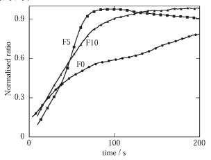
**Figure 5.**Comparative plots of normalised soluble urea concentration versus time for unfilled foam (Fo) and PLSN foams (F5 and F10). Data determined from forced-adiabatic FTIR spectroscopy.
